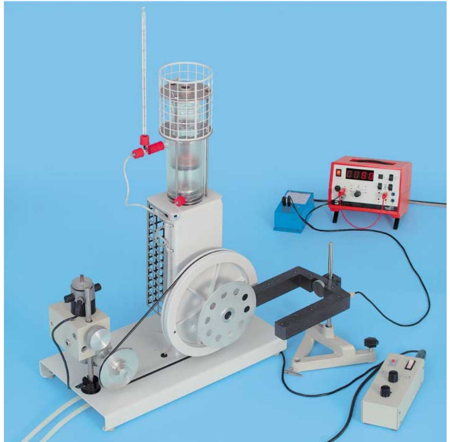
Frictional losses in the hot-air engine (calorific determination) (P 2.7.2.1)
