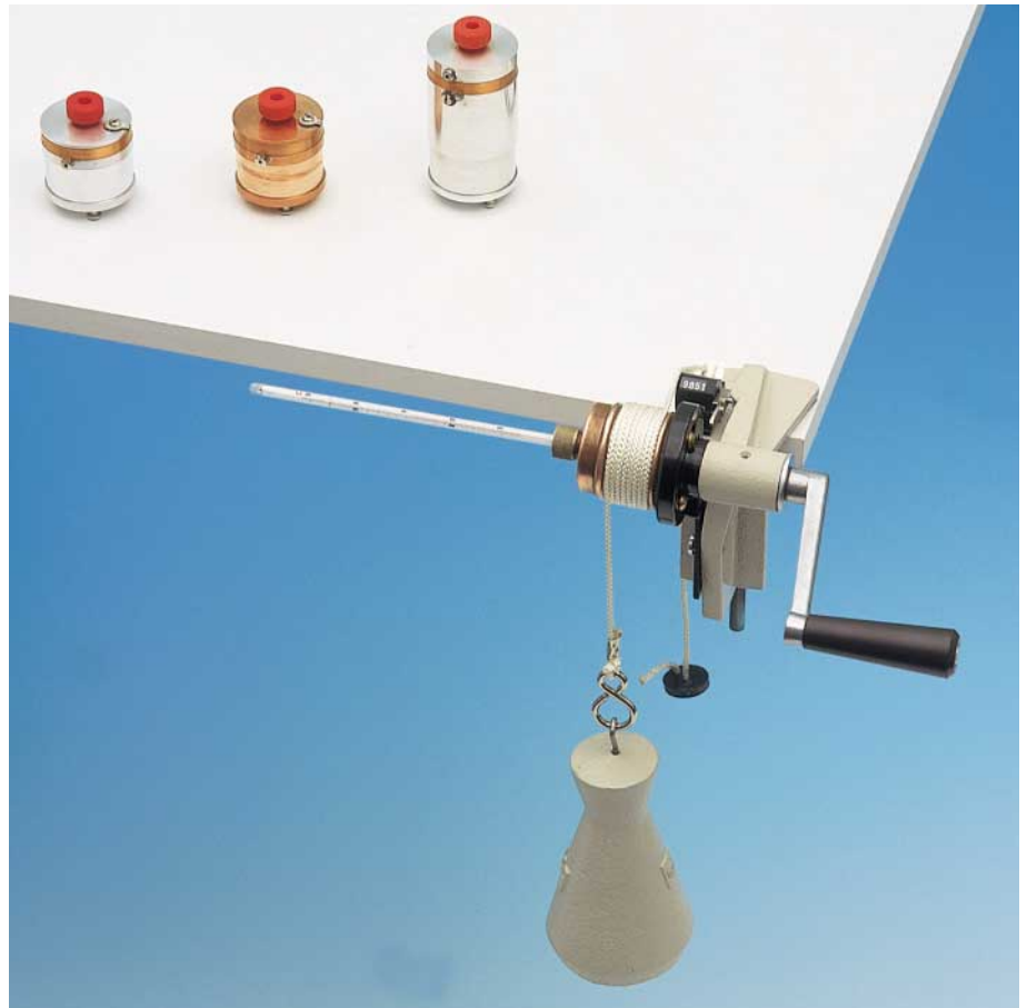
Converting mechanical energy into heat energy – recording and evaluating measured values manually (P 2.3.3.1)
