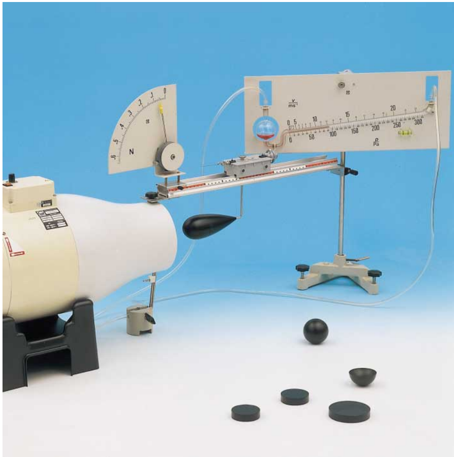
Drag coefficient c_w : relationship between air resistance and body shape - measuring the pressure with the precision manometer (P 1.8.6.2)
