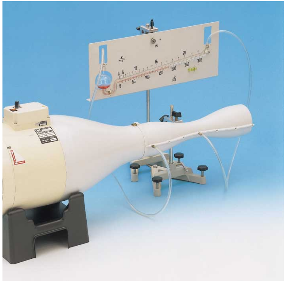
Determining the volume flow with a Venturi tube – measuring the pressure with the precision manometer (P 1.8.5.2)
