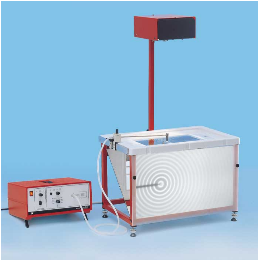
Generating circular water waves (P 1.6.4.1)
