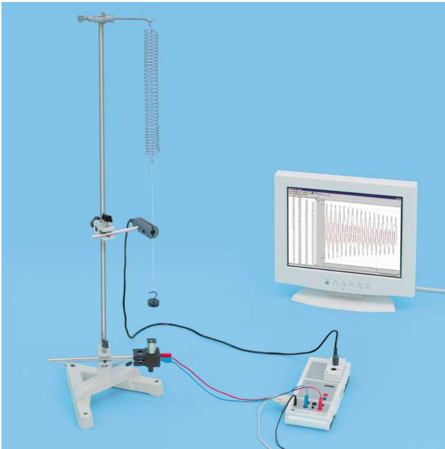
Oscillation of a spring pendulum – recording path, velocity and acceleration with CASSY (P 1.5.2.1)
