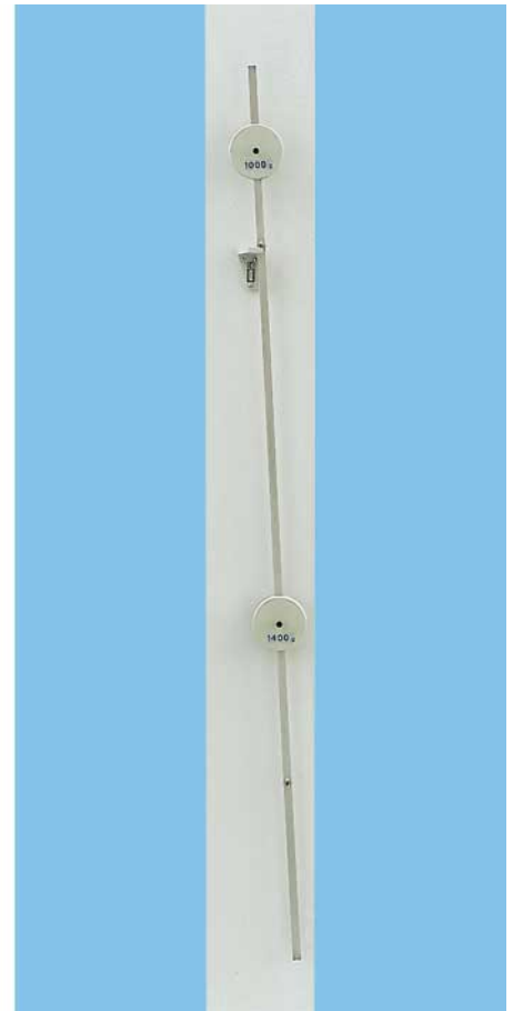
Determining the gravitational acceleration with a reversible pendulum (P 1.5.1.2)
