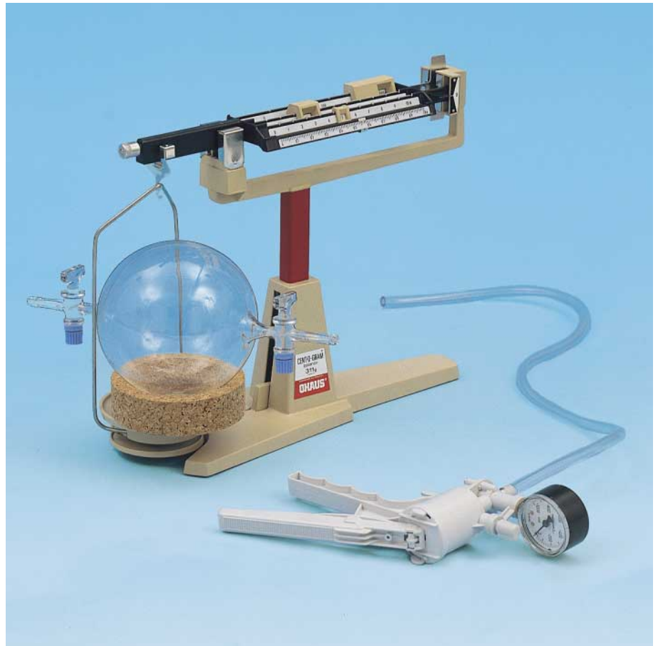
Determining the density of air (P 1.1.2.4)
