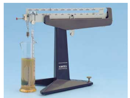
Determining the density of liquids using the Mohr density balance (P 1.1.2.2)
