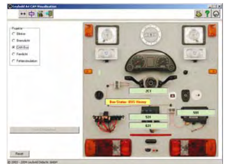
Displaying CAN bus processes on the PC with CAN bus software
