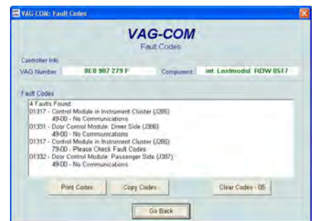
Reading out the fault memory via the diagnose bus
